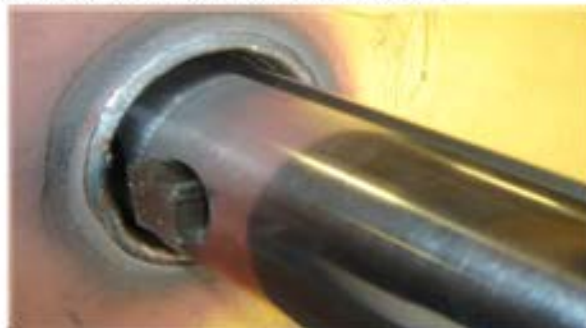
#6. Slide boring bar back through supports and machine bore to size
